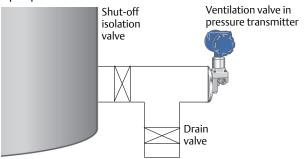
Shut-off isolation and drain valves used for zero calibration of the pressure transmitter.
